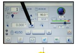
13. Press and hold Bend pedal  $\checkmark$  or  $\vdash$  icon to initiate the bend.
