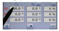
4. Enter desired bend angle, springback and speed setting to complete each line and select OK to enter.
