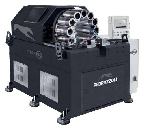
The Stern Brown 160 end former is equipped with Pedrazzoli IMS (Intelligent Motion Software) developed for controlling end forming operations. Software allows operator to visualize part, create, copy and execute program via touchscreen.
