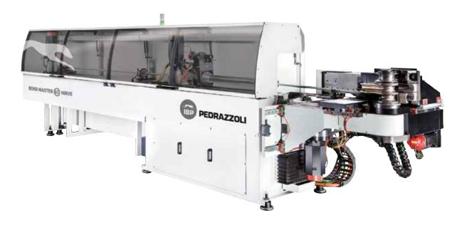
Elevate your metal bending mastery with the Pedrazzoli Bend Master 65, boasting an innovative electric axis control that seamlessly orchestrates clockwise and counter-clockwise bends within a single cycle. Unlock limitless possibilities with the ingenious multi-stack tooling design, engineered to craft bends of impeccable precision in both fixed and variable radii. Crafted from the pinnacle of high-grade steel, the machine's robust framework ensures unwavering performance.
