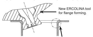
Thickness of material in area of flange radius may be increased. Gain in material at flange radius improves structural integrity.
