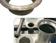
Ercolina's EFB uniformly cold forms a variety of materials including stainless, steel, copper and aluminum to 90° flanges in tubes with maximum wall thickness of .1875".
