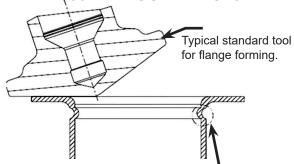
Main defect: collapsing of material around flange collar. Reduced tube diameter results in flow restriction.
