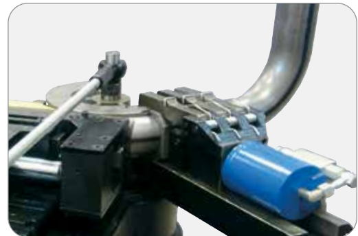
Patented finger style (FST) clamping system minimizes clamping area.
