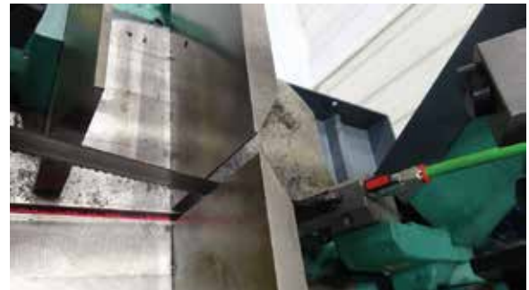
Laser pointer for cutting position
