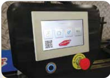
Easy touch screen bend angle programming.
