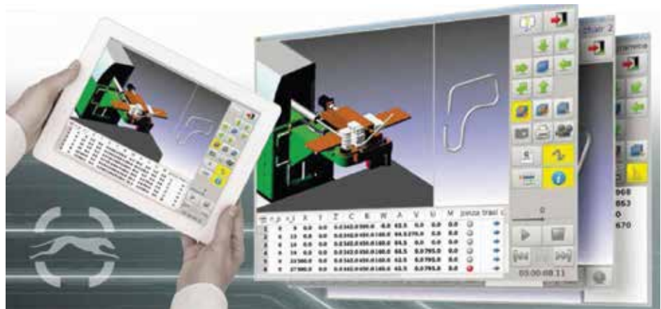
Simulation mode immediately analyzes work piece feasibility, optimizes production time and advises of possible interference.
