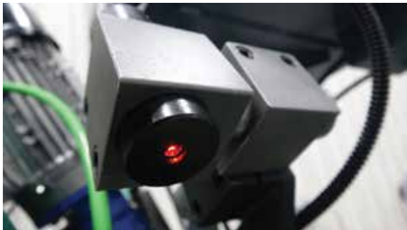
Laser pointer for cutting position
