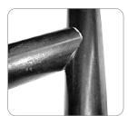
Notch angles to 60° in pipe or tube up to 3" in seconds, to a gap free fit ready for welding.
