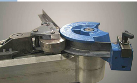
Ercolina rotary draw bender with modified tooling and fabricated roller pressure die to support legs.
