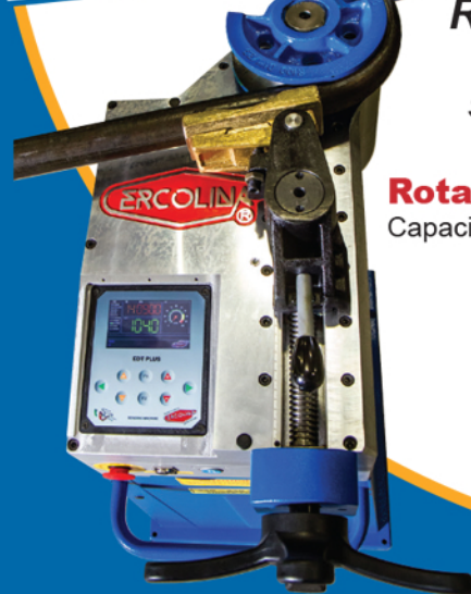
Ercolina rotary draw bender with modified tooling and fabricated roller pressure die to support legs.
