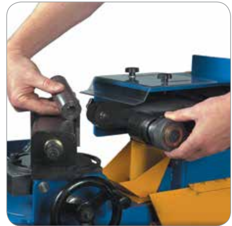
Patented quick-change roller system
