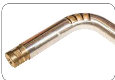
2" Stainless Steel .065wall – 3" CLR Cutaway to show mandrel
